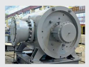
Unified body of Centrifugal Compressor for T25
