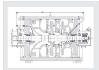
Centrifugal Compressor for GPU-25 "Ladoga", plan
