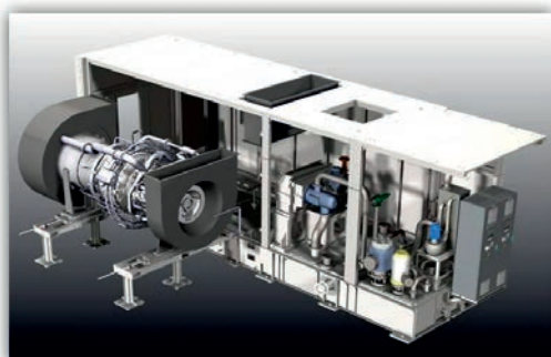
Rolling-Out of the Entire Turbounit
