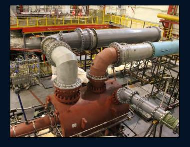
The mixed refrigerant compressor was successfully tested at Nevskiy facility and confirmed contractual specifications.
