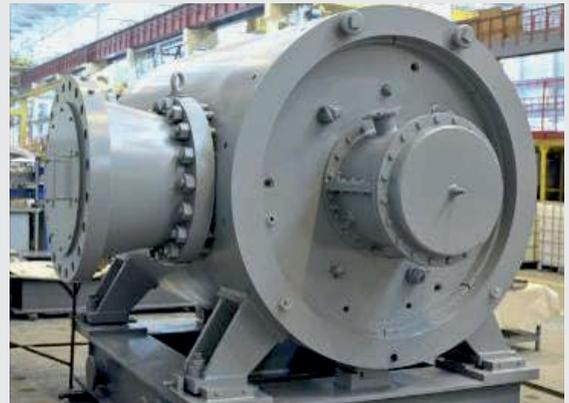
Unified body of Centrifugal Compressor for T25
