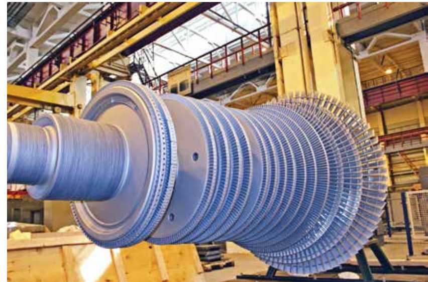
K-22-90-2M Turbine Rotor
