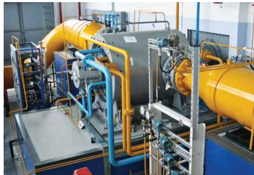
220-11-1SMP centrifugal compressor at Volodino compressor station
