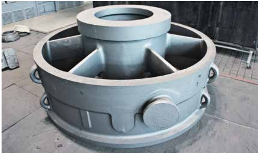
Exhaust Plenum of the LP Turbine
