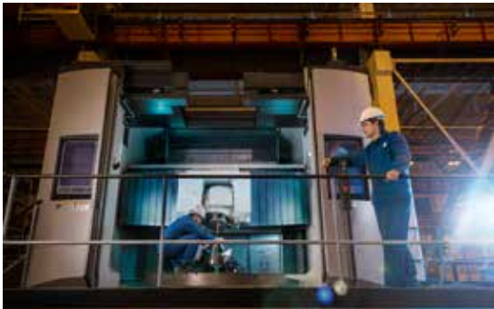
Okuma five-coordinate machining center
