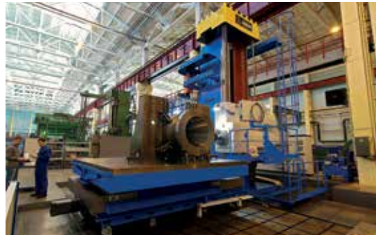
Skoda machine for casings and large-size parts machining
