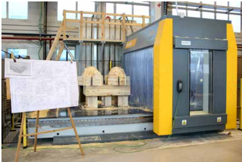
Dinamic FC 4000 CNC 5-coordinate machine to manufacture patterns
