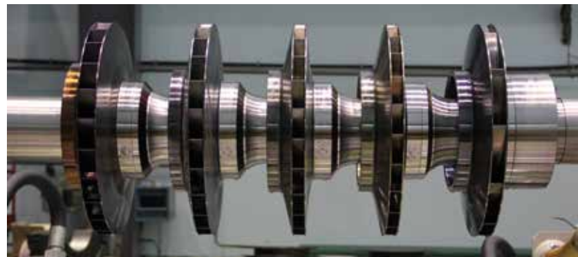
Rotor 155 of the replaceable flow passage on the balancing machine Shenk
