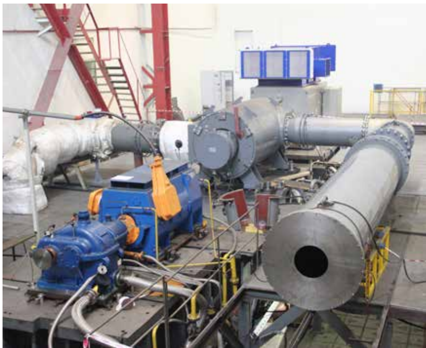
295 Replaceable Flow Passage on the test bench
