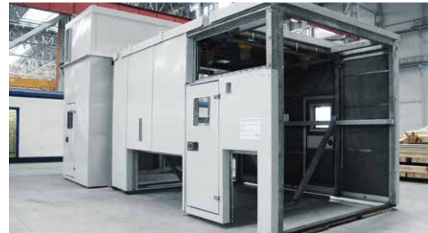
GTU heat-and-noise insulating enclosure
