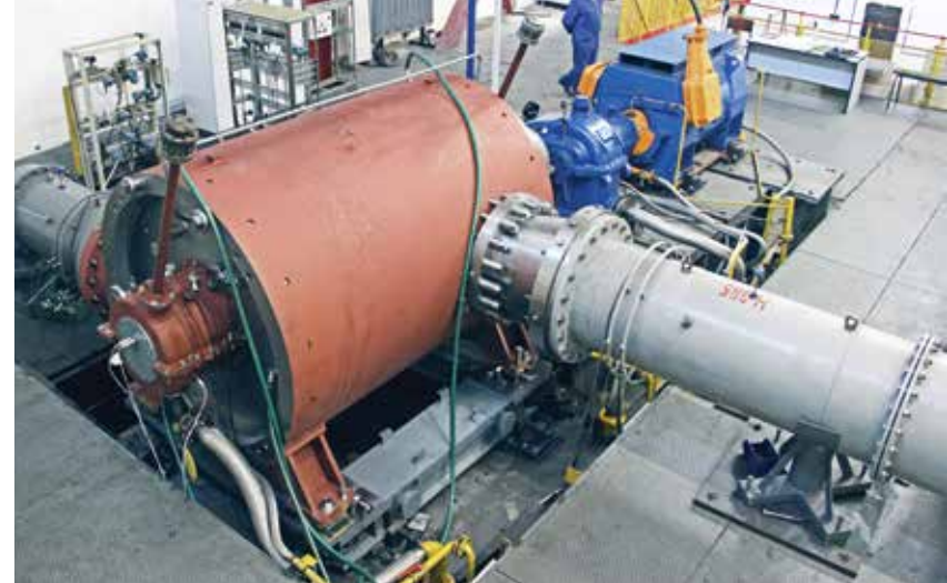
Centrifugal Compressor test bench
