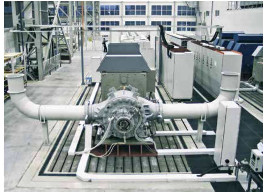
Test bench for Electrically-Driven Gas Pumping Unit (EGPU)
