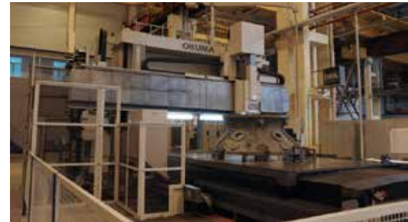
Okuma portal-type machining center
