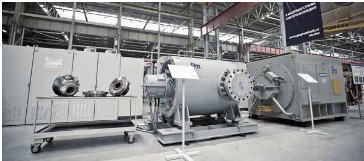
Electrically Driven gas-pumping unit
