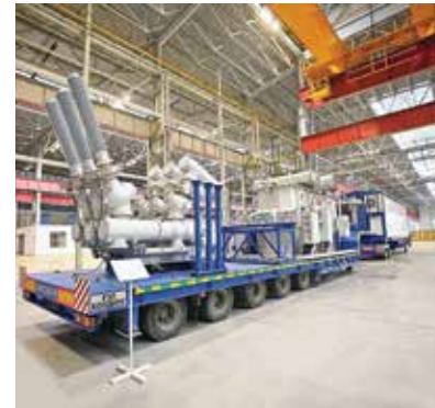
Modular mobile substation (MMS)
