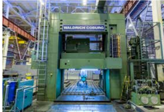
Coburg machine for casings and large-size parts machining
