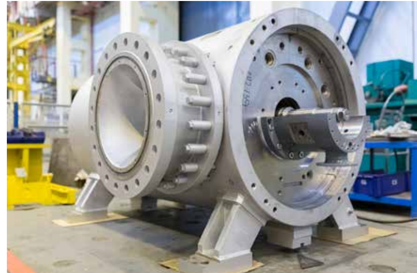
Unified body of Centrifugal Compressor for T25
