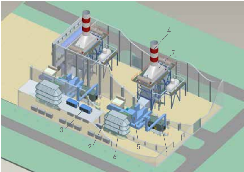
Configuration of the main equipment for GTP – CHPP (Central Heating and Power Plant)
