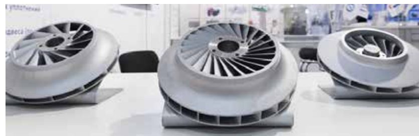
Integrally-machined axial-radial impellers with 3D blades
