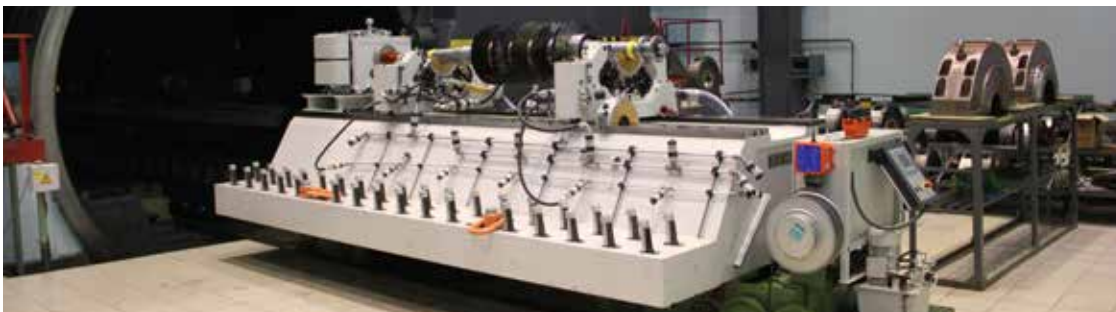
Shenk high-speed balancing and overspeed facility
