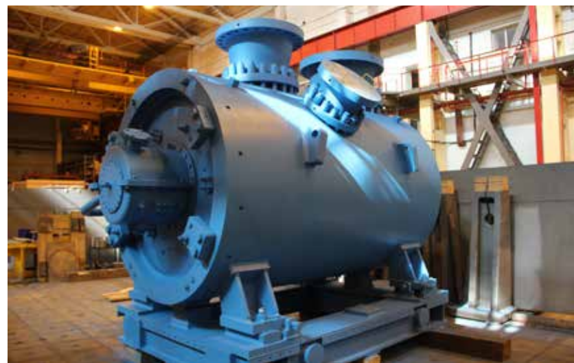
Mixed refrigerant centrifugal compressor K905-71-1C
