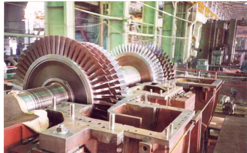
Rotor of top-pressure recovery turbine TPRT 25
