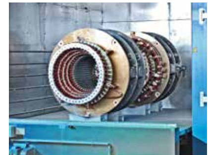
Impregnation of electric motor stators
