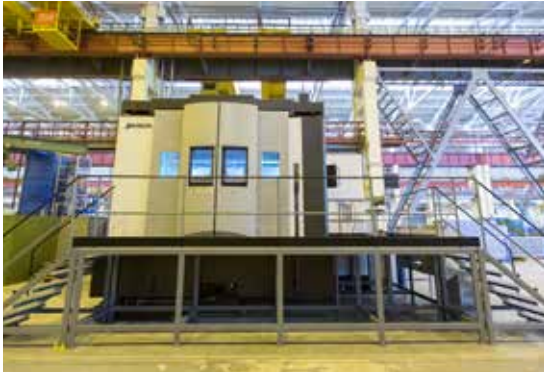
Okuma five-coordinate machining center
