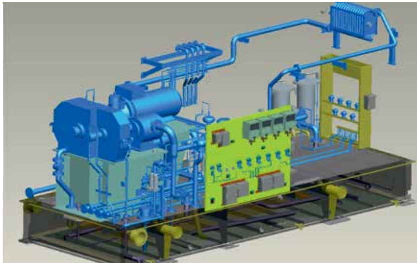
MS5002E auxiliary base plate, 3D-model
