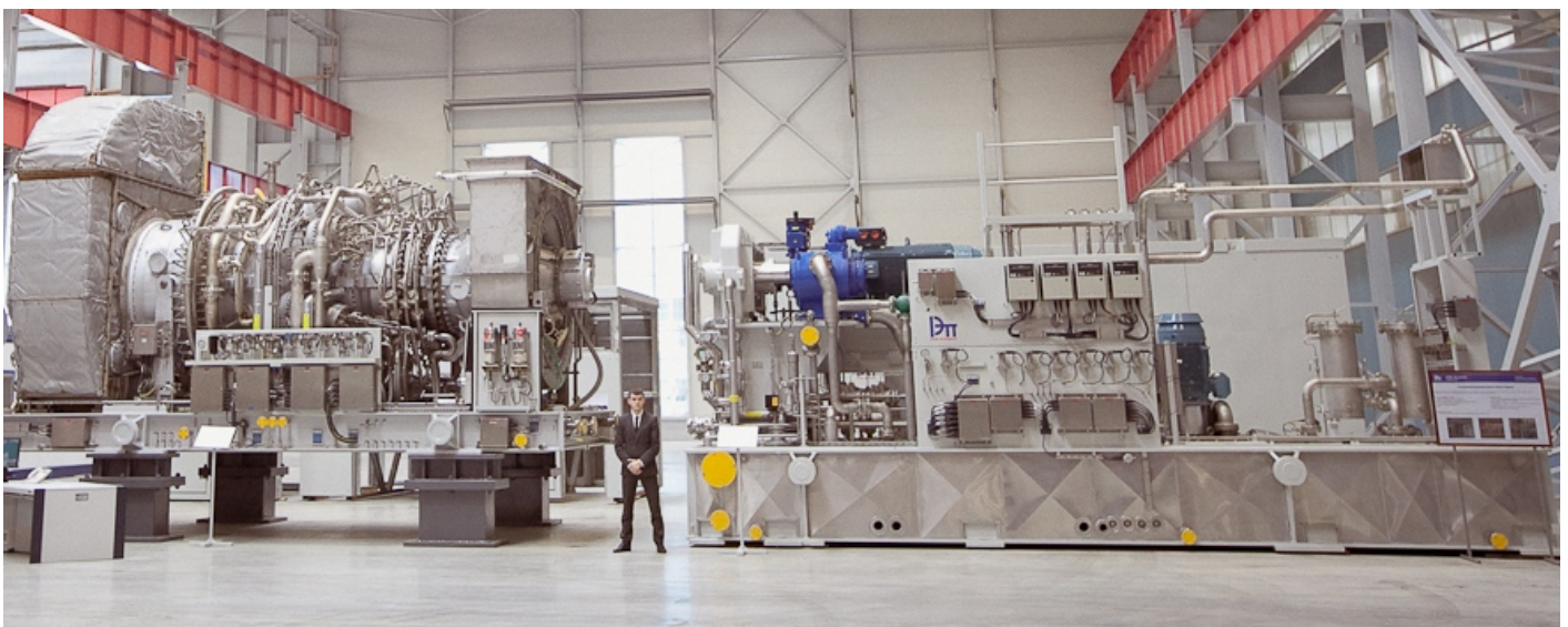
The GTE module with inlet/exhaust ducts (on the left) and auxiliary base plate (on the right) on the REP Holding production site
