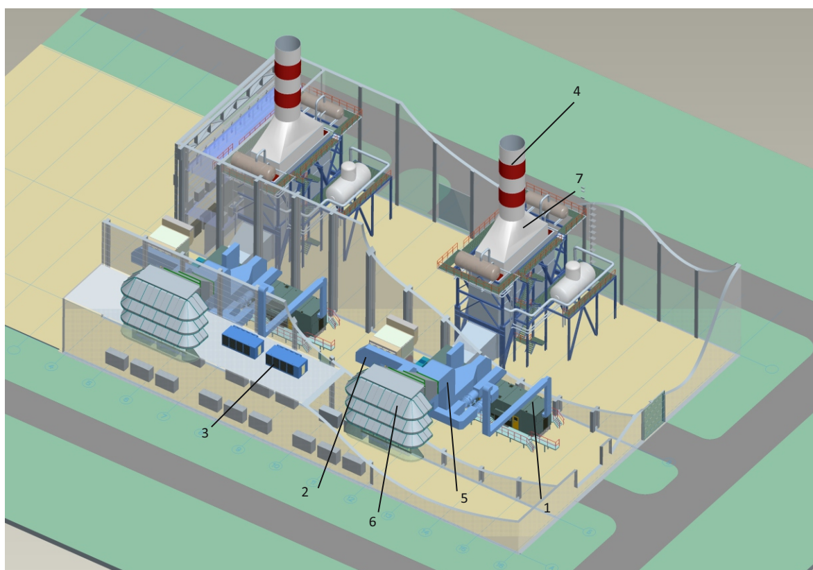
Configuration of the main equipment for GTU – CHPP (Central Heating and Power Plant)
